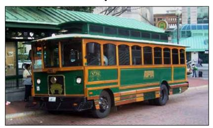
A tourist trolley, also called a road trolley, is a rubber-tired bus, which is made to resemble an old-style streetcar. The name refers to the American English usage of the word trolley to mean an electric streetcar. As these vehicles are not actually trolleys, and to avoid confusion with trolley buses, the American Public Transportation Association (APTA) refers to them as "trolley-replica buses"
