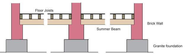
Double building structure cross section
